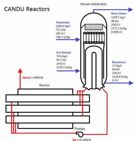
Figure 1. Typical CANDU thermal cycle
